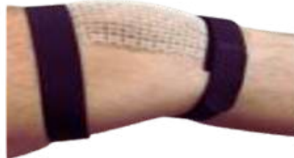
A mesh, featuring anisotropic mechanics and showing the ability to conform to a knee.
