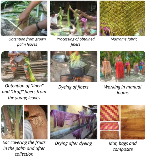
The obtention of Palm fibers, processing, and manufacture of final products (Pennas, et al., 2019)
