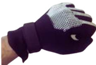
The mesh is sewn onto a glove and, this mesh-enhanced glove exerts a restoring force on the fingers when the fist is clenched (Xiao & Kan, 2022)
